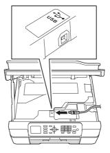
Carefully guide the USB cable into the cable channel and out the back of the machine.
